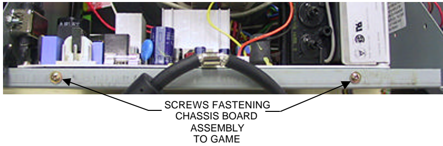
FIGURE 5 - FORCE CLASSIC - CHASSIS BOARD MOUNTING TRAY
